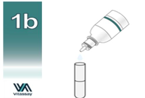
Add 13 drops of Reagent into a testing tube.
