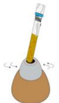
Shake the sample dilution vial with diluent+sample. Use a vortex. Centrifuge.
